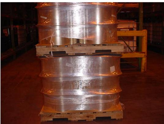
*Heavy weight rolls are being shipped on pallets doubled stacked using a Grip Pad between the two pallets*
